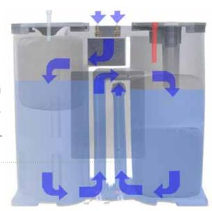
Following this process, the oil remains permanently bound in the high-performance filter elements. Due to the multi-stage arrangement of the filter stages, a residual oil content of < 10 mg/m3 can be ensured even with emulsified condensates.
