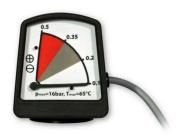
Differential pressure gauges FAD01C with potential free alarm contact allow to hook up the differential pressure control of the pre- and after-filter to the common alarm message of each dryer. To avoid a false error report due to start-up conditions or short-time peaks, an alarm delay can be set in the dryer control unit. The alarm message then will just be generated, if a too high differential pressure was indicated during the entire delay time interval.
