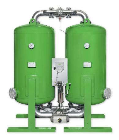
This amount of compressed air is expanded to atmospheric pressure and is led through the vessel to regenerate the desiccant. The dried, decompressed air is extremely moisture-subsaturated and thus extracts the moisture stored in the desiccant and discharges it to the atmosphere via a silencer (heatless regeneration).
