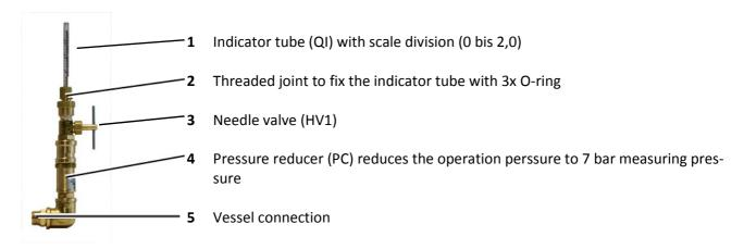
The measuring principle is as follows: For the duration of the measurement, the needle valve (3) is opened so that a pressure-reduced partial flow of purified compressed air is fed through the indicator tube (1). The indicator tube is secured by means of a union nut (2).
