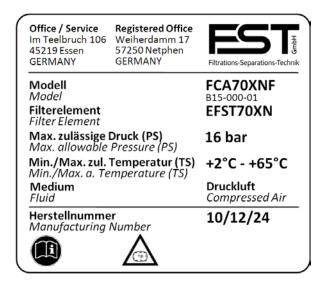
Type plate of the filter on the filter housing (example: FCA70XNF)
